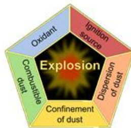
Fig. 1 – Pentagon of ignition to combustible dusts
